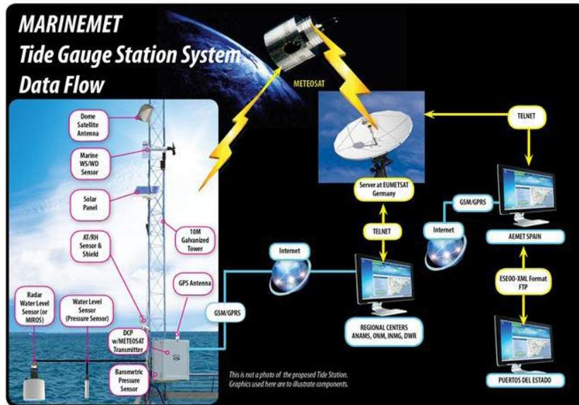
**Figure 4:** The Marine Automatic Weather Station System Data Flow in the Marinemet project as proposed by the contracted supplier. This Project will use a similar setup of equipment for a new station and data adapted to the needs of end users and ONM.
